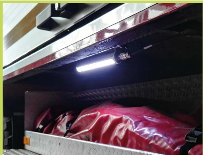
AmbitLED - Additional lighting on the fire engine
